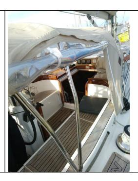
The exposed vertical bars can have protecting covers fitted.
